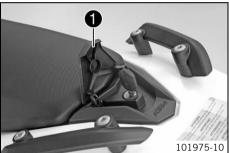
Lift the cover of filler cap 1 and insert the ignition key.
