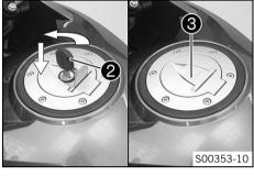
Press down the filler cap and turn back ignition key 2 until the fuel tank lock locks.
