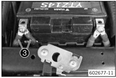
Disconnect the negative cable 3 of the battery to avoid damage to the motorcycle's electronics.
