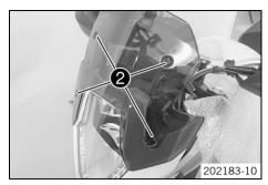
Remove the film from the headlight. Position the screen. Mount and tighten screws 2.
