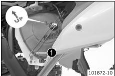
Insert both parts together, position them, and fasten them using air filter holder 1.
