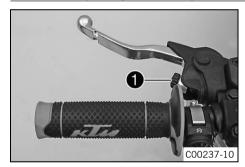
Adjust the basic setting of the clutch lever to your hand size by turning adjusting screw 1.
