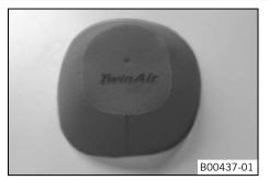
Fit a waterproofing device on the air filter.
