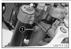
The steering lock ① is fitted on the left of the steering head. The steering lock is used to lock the steering. Steering, and therefore riding, is no longer possible.
