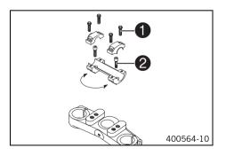
Remove the screws 1. Take off the handlebar clamps. Remove the handlebar and lay it to one side.
