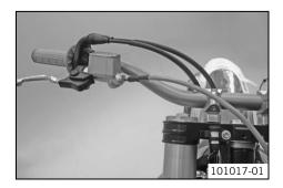
Position FI warning lamp with holder (3). Mount and tighten screw.
