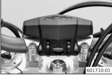
Secure the handlebar cushion with two cable binders.
