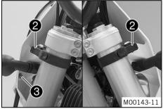
Position the headlight mask and fix it with rubber straps **2**.
