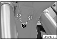
Mount and tighten screws 2.
