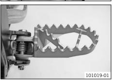
Mount the footrests with the springs and bolts. Secure the bolts using the washers and pins.
