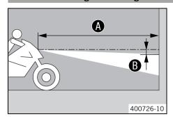
Position the vehicle upright on a horizontal surface in front of a light wall and make a mark at the height of the center of the low beam headlight.
