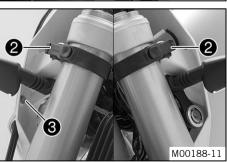
Position the headlight mask and fix it with rubber straps **2**.
