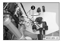
Detach electrical plug-in connector (3) and take off the headlight mask with the headlight.
