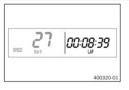
In the  $\ensuremath{\textbf{LAP}}$  display mode, up to 10 lap times can be timed with the stop watch.
