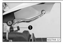
Check the free travel of the hand brake lever. (\* p. 77)
