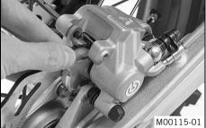
Check that leaf spring **(5)** in the brake caliper and sliding plate **(6)** in the brake caliper support are seated correctly.
