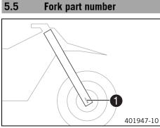
The fork part number **①** is stamped on the inner side of the fork stub.
