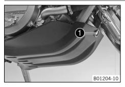
Turn quick release ① counterclockwise until it disengages. Remove the engine guard.
