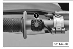
The kill switch **1** is fitted on the left side of the handlebar.
