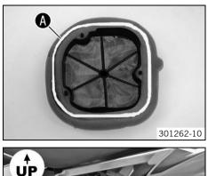
Installing the air filter 🔌
