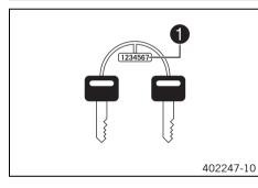
The key number 1 for the steering lock is stamped onto the key connector.
