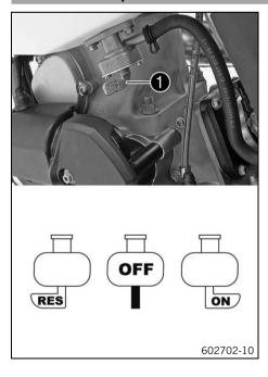
The fuel tap is on the left side of the fuel tank.
