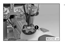
Press release button  $oldsymbol{1}$ , turn the filler cap counterclockwise and lift it free.
