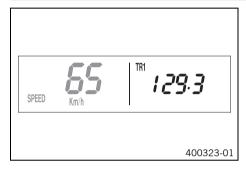
**TR1** (trip master 1) runs constantly and counts up to 999.9. You can use it to measure trips or the distance between refueling stops. **TR1** is coupled with **A1** (average speed 1) and **S1** (stop watch 1).
