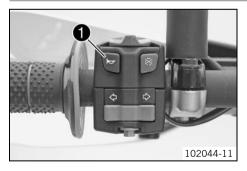
The horn button **()** is fitted on the left side of the handlebar. **Possible states**
