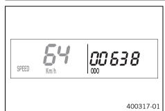
Repeatedly press the button H briefly until **ODO** appears at the bottom right of the display.
