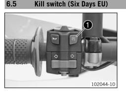
The kill switch **1** is fitted on the left side of the handlebar.
