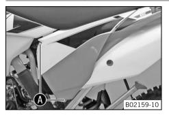
Pull off the air filter box lid in area 🚯 sideways and remove it toward the front.
