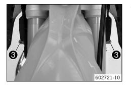
Pull both spoilers off of the sides of the radiator bracket **3** and lift off the fuel tank.
