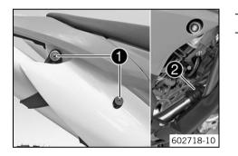
Installing the main silencer
