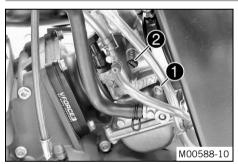
Screw idle air adjusting screw 1 all the way in.
