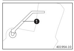
Kick starter **①** is fitted on the right side of the engine. The top part of the kick starter pivots.
