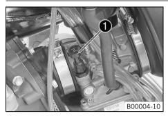
The choke lever **①** is fitted on the left side of the carburetor. Activating the choke function frees an opening in the carburetor through which the
