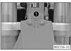
Installing the front fender
