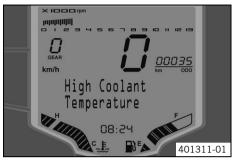
**High Coolant Temperature** appears on the info display if the coolant temperature rises above the specified value.
