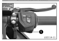
The electric starter button **1** is fitted on the right side of the handlebar.
