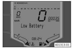
Low Battery appears on the info display if the battery voltage falls below the specified value.
