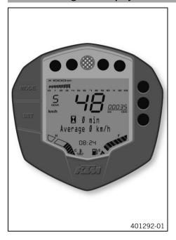
The filling level display consists of 9 bars. The more bars are lit, the more fuel is in the fuel tank.
