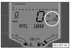
✓ The display **RPM 1** goes out and the set speed is stored.
