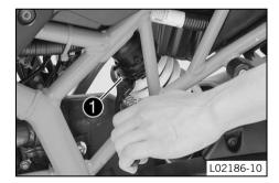
Set the spring preload by turning adjusting ring using the hook wrench from the tool set.
