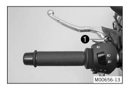
Adjust the basic position of the clutch lever to your hand size by turning adjusting screw 1.
