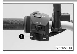
The horn button 1 is fitted on the left side of the handlebar.
