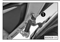
The seat lock 1 is located on the left side of the vehicle. It can be locked with the ignition key.
