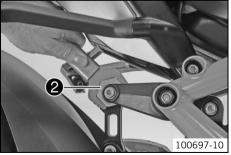
Turn eccentric shaft **2** to the desired position using the tool from the tool set. Guideline
