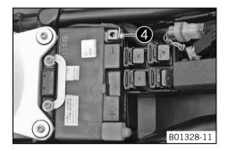
Position the negative cable 4 and mount and tighten the screw.
