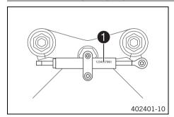
The steering damper part number 1 is stamped on the top of the steering damper.
