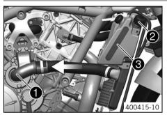
The water pump with a 3D water pump wheel
