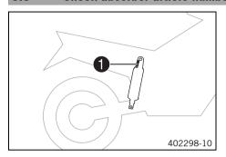
The shock absorber part number **1** is stamped on the top of the shock absorber above the adjusting ring towards the rear.
