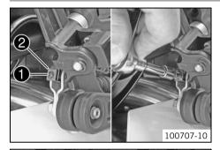
Use the tool to press in the anti-rotation lock 2, then turn the piston rod 1.
