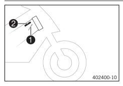
The vehicle identification number **1** is stamped on the frame behind the steering head on the right.
