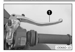
The hand brake lever is fitted on the right side of the handlebar. The hand brake lever operates the front brake.
