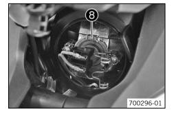
Position the new headlight bulb in the headlight housing.
