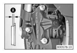
Check all brake linings on both brake calipers to ensure they have minimum thickness A.
