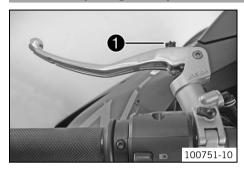
Adjust the basic setting of the clutch lever to your hand size by turning adjusting screw 1.
