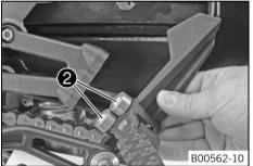
Position the footrest bracket with spacers 2 and screws.
