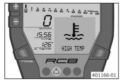
**HIGH TEMP** appears on the info display if the coolant temperature rises above the specified value.
