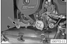
Mount and tighten the oil drain plugs with the magnets, O-rings, and oil screens.
