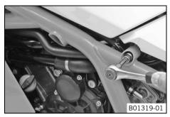
Mount the screws with the washer on the left and right sides of the vehicle but do not tighten yet.
