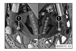
Turn adjusting screws 1 clockwise to the stop.
