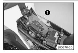
The tool set **1** is in the storage compartment under the seat.
