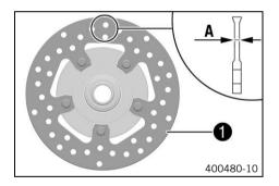
Check the thickness of the brake disc in several places to see if it conforms to measurement (A).
