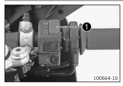
The emergency OFF switch 1 is installed on the right side of the handlebar.
