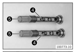
Thoroughly clean magnets 4 and oil screens 5 of the oil drain plugs.
