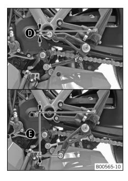
Adjust the shift lever by turning the shift rod.
