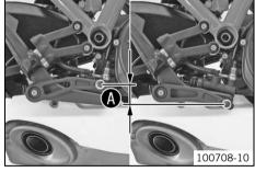
Check the foot brake lever setting.
