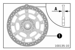
Check the thickness of the brake disc in several places to see if it is within the specified wear tolerance A.
