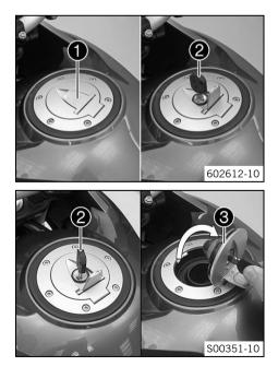
Lift cover 1 of the filler cap and insert ignition key 2 in the fuel tank lock.
