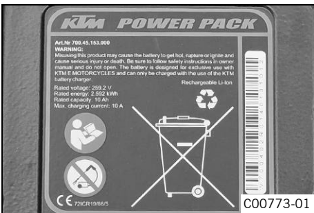
Rechargeable lithium-ion battery
