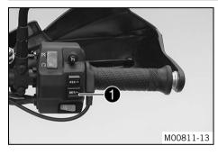
The lower button **1** of the cruise control system is fitted on the right side of the combination switch.
