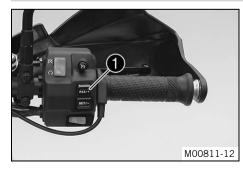
The upper button **1** of the cruise control system is fitted on the right side of the combination switch.
