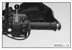
The emergency OFF switch (1) is fitted on the right side of the combination switch.
