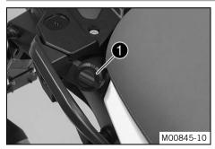
The passenger seat heating switch **()** is located next to the right grab handle.
