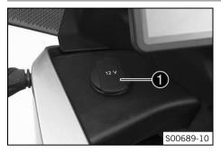
Socket **①** for electrical accessories is fitted to the left of the combination instrument. It is connected to permanent positive and fuse-protected.
