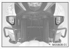
The cornering headlight is located to the left and the right in the side cover.
