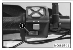
The horn button **()** is fitted on the combination switch on the left.
