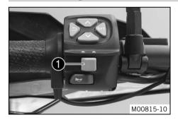
The turn signal switch **1** is fitted on the combination switch on the left.
