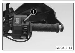
The switch for the cruise control system is fitted on the right side of the combination switch.
