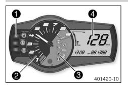
The combination instrument is installed in front of the handlebar.
