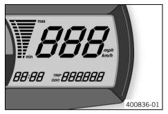
When the ignition is switched on, all display segments light up for one second as a function check.
