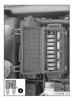
Remove the defective fuse
