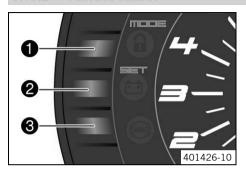
You can change the display mode with the **MODE** button **1**. Possible display modes are distance traveled **(ODO)**, trip master 1 **(TRIP 1)** and trip master 2 **(TRIP 2)**.
