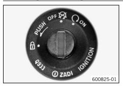
The ignition/steering lock 1 is located in front of the seat.
