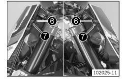
Position brake line guides **(6)**. Mount and tighten screws **(7)**. Guideline
