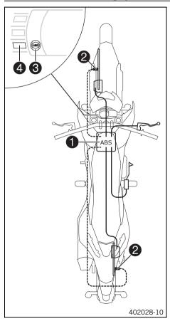
The <u>ABS</u> unit **1**, which consists of a hydraulic unit, ABS control unit, and return pump, is installed under the seat. A wheel speed sensor **2** is located at both the front and the rear wheel.
