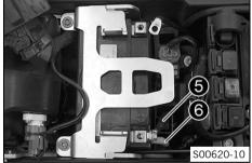
Disconnect the ABS connection cable 6 and positive cable 6 from the battery.
