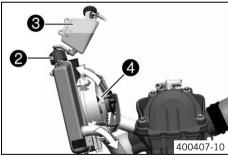
Cooling takes place by means of the air stream and a radiator fan 4, which is controlled by a thermoswitch.
