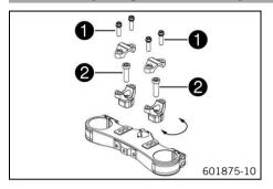
Remove screws 1. Take off the handlebar clamps. Remove the handlebar and lay it to one side.
