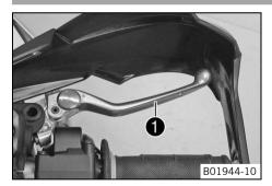
The hand break lever **1** is fitted on the right side of the handlebar. The hand brake lever operates the front brake.
