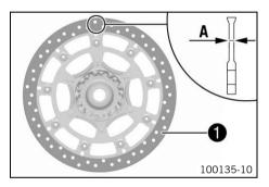
Check the thickness of the front and rear brake discs in several places to ensure that it conforms to measurement A.
