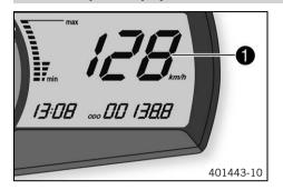
The speed **1** is shown in kilometers per hour **km/h** or in miles per hour **mph**.
