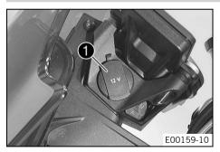
Socket **1** for electrical accessories is mounted on the left side of the instrument support. It is connected to the permanent positive and is fuse-protected.
