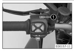
The hazard warning flasher switch **1** is fitted on the combination switch on the left. The hazard warning flasher is used to indicate emergency situations.
