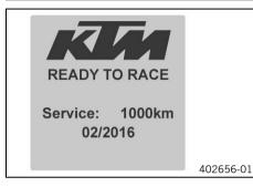
The matrix display is controlled using the <u>menu switch</u> (P p. 29). After the ignition is switched on, the display shows when the <u>next service</u> (P p. 50) is due. If the General warning lamp  $\blacksquare$  lights up among the <u>indicator lamps</u> (P p. 47), the corresponding message appears in the matrix display. The **Set** button is used to confirm receipt of the information and the message is cleared.
