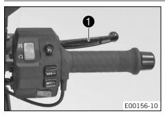
The hand brake lever **1** is fitted on the right side of the handlebar. The front brake is engaged using the hand brake lever.
