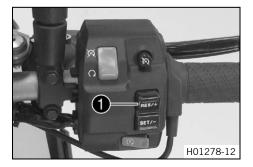
Upper button **1** of the cruise control system is fitted on the right side of the combination switch.
