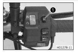
Switch **1** for the cruise control system is fitted on the right of the combination switch.
