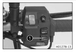
Lower button **1** of the cruise control system is fitted on the right side of the combination switch.
