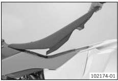
Hook in the front of the seat at the collar bushing of the fuel tank, lower it at the rear and simultaneously push it forward.
