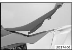
Raise the rear of the seat, push the seat back, and lift it off.
