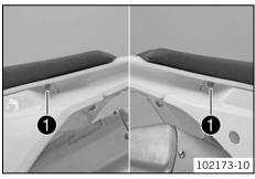
Mount and tighten the seat fixing screws ①.
