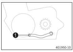
Shift lever **()** is mounted on the left side of the engine.
