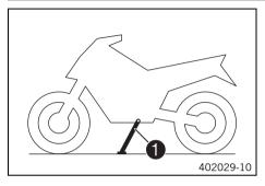
The side stand **1** is on the left side of the vehicle. The side stand is used to park the motorcycle.
