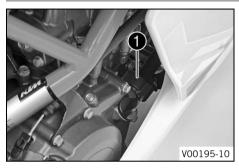
Water pump **①** in the engine circulates the coolant.
