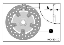
Check the thickness of the front and rear brake discs at multiple points on each brake disc to ensure it is at least thickness (A).
