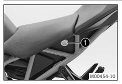
The seat lock **1** is located to the left of the seat. The seat lock can be unlocked using the ignition key.
