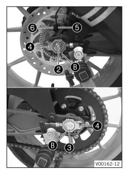
Pull the rear wheel back and mount wheel spindle 3 with the washers and chain adjusters 4.
