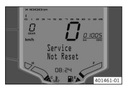
**Service Not Reset** appears on the info display for 10 seconds when the ignition is switched on and the distance interval between service appointments has been exceeded or the service interval display was not reset during a service appointment.
