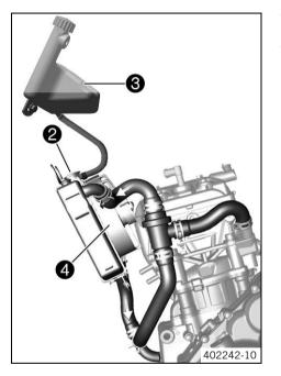
The coolant is cooled by the air stream and a radiator fan (4), which is controlled by a thermoswitch.
