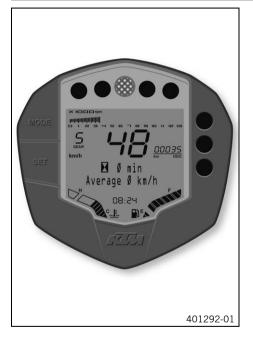
The temperature display consists of 13 bars. The more bars that light up, the hotter the coolant. When all bars light up, the following warning note appears on the info display: **High Coolant Temperature**.
