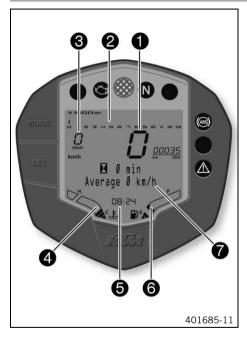
The speed 1 is shown in kilometers per hour **km/h** or in miles per hour **mph**. The tachometer 2 shows the engine speed in revolutions per minute. The gear display 3 shows the engaged gear. The coolant temperature appears in segment 4. The time appears in segment 5. The filling level in the fuel tank is displaced in segment 6. The info display 7 shows additional information.
