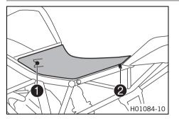
Attach recesses **1** on the front rider's seat to the fuel tank, push the front rider's seat forward, and lower at the rear.
