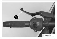
The clutch lever **1** is fitted on the left side of the handlebar.
