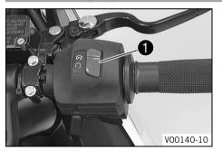
The emergency OFF switch **()** is fitted on the right side of the handlebar.
