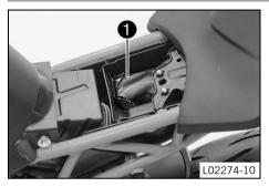
The tool set **1** is in the storage compartment under the seat.
