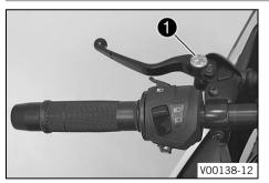
Adjust the basic position of the clutch lever to your hand size by turning adjusting wheel 1.
