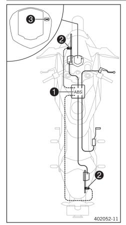
The ABS unit ①, which consists of a hydraulic unit, ABS control unit, and return pump, is installed under the seat. One wheel speed sensor ② is located in each case on the front and the rear wheel.
