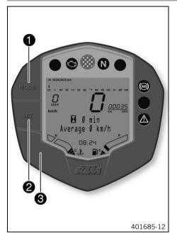
You can change the display mode with the **MODE** button **1**. Possible display modes are total distance traveled (**TRIP 1**), distance 1 (**ODO**) and
