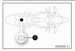
Diagnostics connector **1** is located under the front rider's seat.
