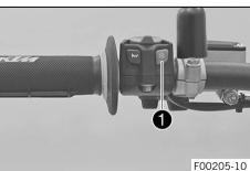
(EU) The kill switch 1 is fitted on the left side of the handlebar.
