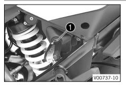
Seat lock **1** is located on the left side of the vehicle under the seat. It can be unlocked using the Race-on key or the black Race-on key.
