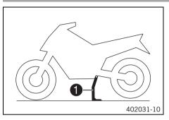
In addition to the side stand, the vehicle is equipped with a center stand (1).
