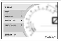
Settings for different loading conditions can be selected in the Load menu. A selection can be made between one-person operation, one-person operation with luggage, two-person operation, and two-person operation with luggage.
