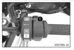
The hazard warning flasher switch  $\mathbf{1}$  is fitted on the right side of the combination switch. The hazard warning flasher is used to indicate emergency situations.
