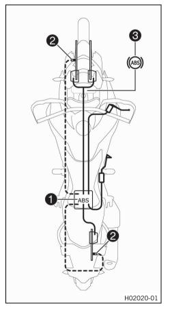
The ABS unit (1), which consists of a hydraulic unit, brake electronics control unit, and return pump, is installed under the seat. One wheel speed sensor (2) is located in each case on the front and the rear wheel.
