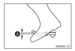
Sit on the vehicle in the riding position and determine distance A between the upper edge of your boot and the shift lever.
