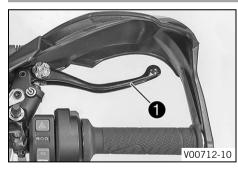
The hand brake lever **1** is fitted on the right side of the handlebar. The hand brake lever is used to activate both the front brake and rear brake at the same time.
