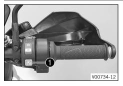
The <u>Race-on button</u> **①** is fitted on the right side of the combination switch.
