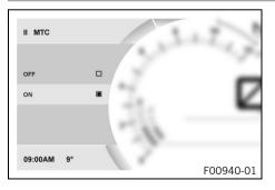
The motorcycle traction control ( $\underline{MTC}$ ) lowers the engine torque in case of loss of traction in the rear wheel. Depending on the motorcycle traction control setting, a slight slip on the rear wheel may be desirable. Example: offroad.
