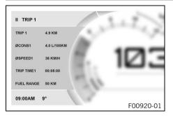
When the menu is closed, the **Quick Selector 1** menu is opened by pressing the **UP** button. Press the **BACK** button to close **Quick Selector 1**.
