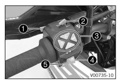
The left combination switch is fitted on the left side of the handlebar.
