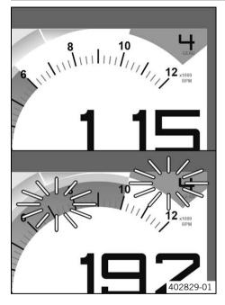
The shift warning light is integrated in the tachometer display.
