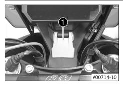
Socket **①** for electrical accessories is fitted in front of the upper triple clamp. It is connected to the permanent positive and is fuse-protected.
