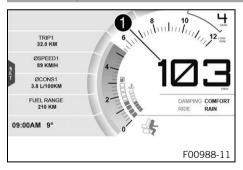
Speed **1** is shown in kilometers per hour **km/h** or in miles per hour **mph**.
