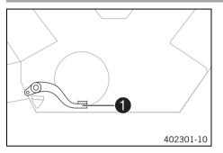
Foot brake lever **①** is located in front of the right footrest. The rear brake is activated using the foot brake lever.
