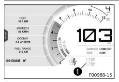
When the seat heating is switched on, the **Heated Seat** symbol appears in the **①** area of the display.
