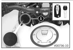
On this vehicle, the ignition/steering lock is replaced by a remote key with transponder (Race-on key (P p. 35)).
