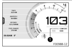
The setting of the spring element damping is shown in the **1** area of the display. The damping can be configured in the **Damping** menu.
