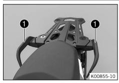
The passenger can hold onto grab handles **①** during the trip.
