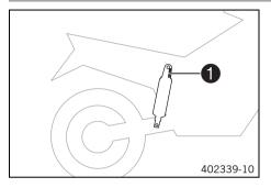
The shock absorber article number ① is stamped on the top of the shock absorber above the adjusting ring towards the engine side.
