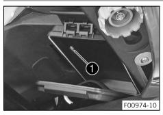
A USB socket **1** is located in the storage compartment for supplying power to external devices.
