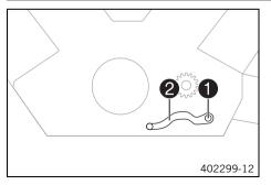
Remove screw **1** with the washers and take off shift lever **2**.
