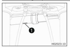
Steering damper article number 1 is embossed on the underside of the steering damper.
