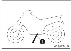
The side stand **①** is located on the left side of the vehicle. The side stand is used for parking the motorcycle.
