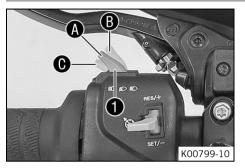
The light switch **1** is fitted on the combination switch on the left.
