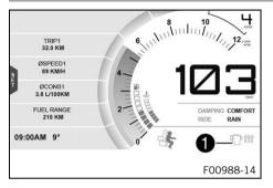
When the heated grip is switched on, the **Heated Grips** symbol appears in the **1** area of the display.
