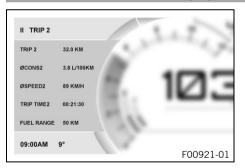
When the menu is closed, the  ${\bf Quick\ Selector\ 2}$  menu is opened by pressing the  ${\bf DOWN}$  button.
