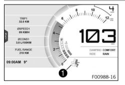
The load condition setting is shown in the **1** area of the display. The payload can be configured in the **Load** menu.
