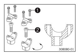
Remove screws ①. Remove the handlebar clamps. Remove the handlebar and lay it to one side.
