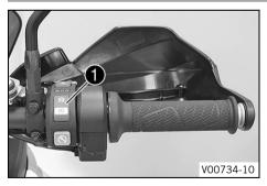
The emergency OFF switch/electric starter button  $\mathbf{1}$  is fitted on the right side of the combination switch.
