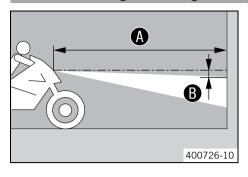
Park the vehicle on a horizontal surface in front of a light-colored wall and make a mark at the height of the center of the low beam headlight.
