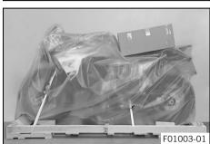
Remove the adhesive tape in the upper area of the motorcycle.
