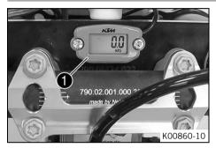
The service hour counter **①** is fitted in front of the handlebar.
