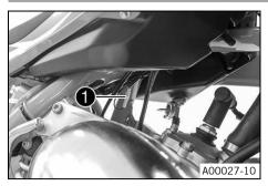
Plug-in connector 1 of the ignition timing map adjustment is located on the frame under the fuel tank.
