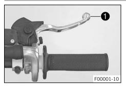
Hand brake lever **1** is fitted on the right side of the handlebar. The front brake is engaged using the hand brake lever.
