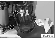
Mount filler cap 1 and turn it clockwise until the fuel tank is tightly closed. Info • Run the fuel tank breather hose **2** without kinks.
