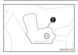
The engine number 1 is embossed on the left side of the engine over the engine sprocket.
