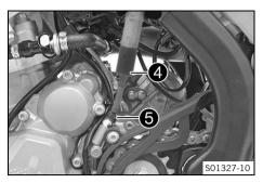
Fill bleeding syringe 4 with the appropriate hydraulic fluid.
