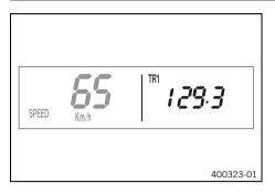
**TR1** (trip master 1) runs constantly and counts up to 999.9. You can use it to measure trips or the distance between refueling stops
