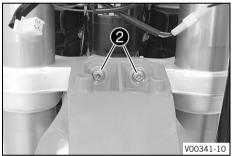
Mount and tighten screws 2.
