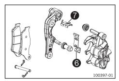
Check that leaf spring 6 in the brake caliper and sliding plate 7 in the brake caliper support are seated correctly.
