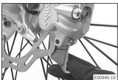
Insert the new brake linings, insert the pin, and mount the cotter pins.
