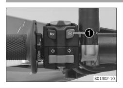
Kill switch **1** is fitted on the left side of the handlebar.
