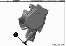
Cold start button **1** is fitted on the bottom of the throttle valve body.
