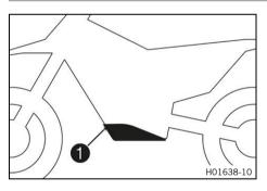
Remove screws 1 and engine guard.
