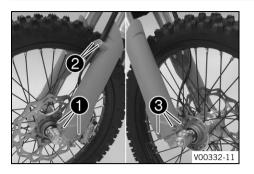
Position the fork protector on the left fork leg. Mount and tighten screws 1.
