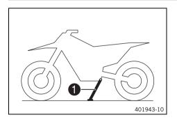
The side stand 1 is attached to the left side of the vehicle.
