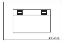
Lithium-ion batteries are far lighter than lead batteries, have a low self-discharge rate, and have more starting power at temperatures over  $15\,^{\circ}\text{C}$  (60 °F). At low temperatures, however, the starting power of lithium-ion batteries drops to below that of lead batteries.
