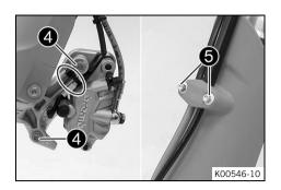
Position the brake caliper, and mount and tighten screws 4. Guideline
