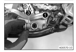
Mount and tighten screw plug 3 with the O-ring.
