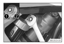
Using an open end wrench, turn adjusting screw 1 clockwise all the way.
