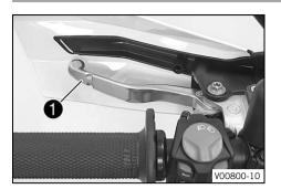
Clutch lever is fitted on the handlebar on the left. The clutch is activated hydraulically and adjusts itself automatically.
