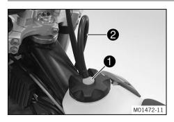
Replace the filler cap and turn clockwise until the release button 1 locks in place.
