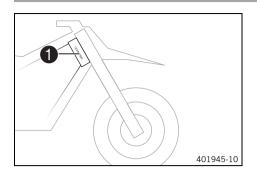
The chassis number **1** is stamped on the steering head on the right.
