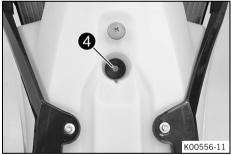
Pull both spoilers off the sides of the radiator bracket and lift off the fuel tank.
