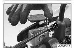
Correct the brake fluid quantity to level **A**. Guideline
