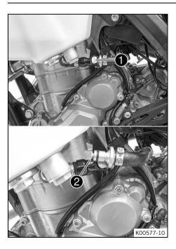
Clean plug-in connection of the fuel line thoroughly with compressed air.
