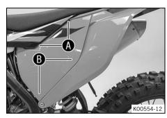
Insert the air filter box cover in area and clip it into area .
