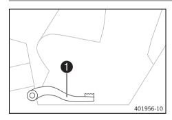
The foot brake lever **1** is attached in front of the right footrest. The foot brake lever is used to activate the rear brake.
