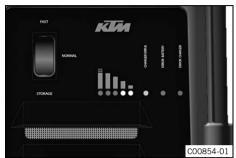
Monitor the charging level of the KTM PowerPack using the LEDs.
