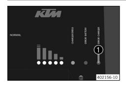
The faults are indicated by LED ① on the battery charger. All of the following blink codes are displayed on the charger and refer to the charger itself.
