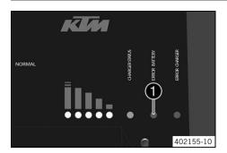
The faults are indicated by LED ① on the battery charger. All of the following blink codes are displayed on the charger and refer to the KTM PowerPack.
