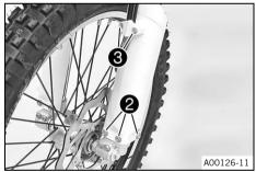
Position the fork protector on the left fork leg. Mount and tighten screws 2.
