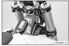
Attach the brake line and wiring harness. Close holder **9**.
