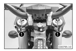
Turn adjusting screws 1 clockwise all the way.
