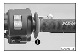
The start button is fitted on the right side of the handlebar. The start button is only enabled when the main switch is switched on.
