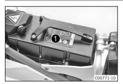
The battery identification number ( $\underline{BIN}$ ) 1 is stamped under the handle of the KTM PowerPack.
