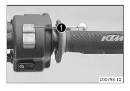
The main switch **1** is attached to the right side of the handlebar. The main switch is also used as an emergency OFF switch.
