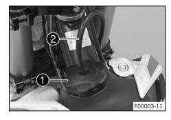
Mount filler cap 1 and turn it clockwise until the fuel tank is tightly closed.
