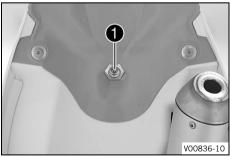
Mount and tighten screw 1 of the seat fixing.
