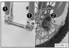
Position the fender. Mount and tighten the screws.
