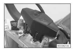
Position the handlebar cushion and secure with cable ties.
