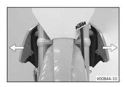
Pull both spoilers off laterally from the radiator bracket and lift off the fuel tank.
