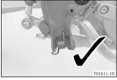
Position the spring in the hole as shown.
