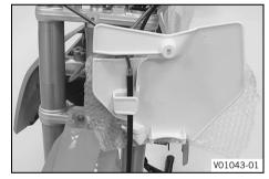
Attach the start number plate to the brake line.
