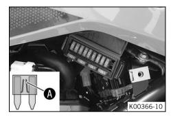
Remove the defective fuse.
