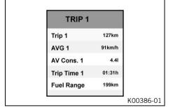
Press the **UP** or **DOWN** button until the "**Trip 1**" menu appears on the display.
