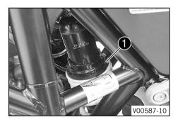
Adjust the spring pretension by turning adjuster ①.
