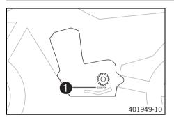
The engine number 1 is located on the left side of the engine under the engine sprocket.
