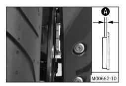
Check the brake linings for minimum thickness  $\mathbf{A}$ .
