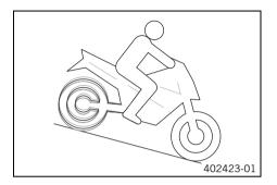
The <u>MSR</u> is an optional auxiliary function of the engine control. If the engine braking effect is too great, the **MSR** prevents the rear wheel from locking.
