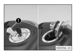
Lift cover 1 of the filler cap and insert the ignition key in the lock.
