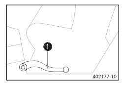
Foot brake lever **1** is located in front of the right footrest. The rear brake is engaged with the foot brake lever.
