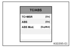
The traction control ( $\underline{\text{TC}}$  ( $\boxtimes$  p. 189)) lowers the engine torque in case of loss of traction in the rear wheel. Depending on the traction control setting, a slight slip on the rear wheel may be desirable.
