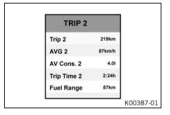
Press the **UP** or **DOWN** button until the "**Trip 2**" menu appears on the display.
