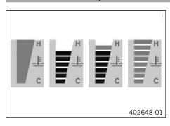
The temperature display consists of 8 bars. The more bars that light up, the hotter the coolant.
