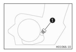
Mount and tighten oil filler plug with the O-ring.
