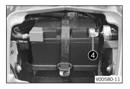
Connect negative cable 4 to the battery.
