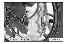
Position wheel speed sensor 4 in the drill hole. Mount and tighten screw 5.
