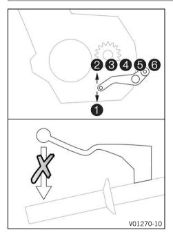
If the <u>quickshifter +</u> is activated, you can shift up and down without actuating the clutch.
