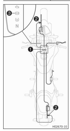
ABS unit ①, which consists of a hydraulic unit, ABS control unit, and return pump, is installed under the fuel tank. One wheel speed sensor ② is located in each case on the front and the rear wheel.
