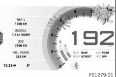
The shift warning light is integrated in the tachometer display. In the **Shift Light** menu, the engine speed for the shift warning light can be set. The shift warning light is always active during the running-in phase (up to 1,000 km / 621 mi). The shift warning light can only be deactivated, and the values for **RPM1** and **RPM2** can only be adjusted after this. The shift warning light lights up red at **RPM1** and flashes red at **RPM2**.
