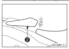
Attach the hooks on the passenger seat 1 to the hanger on the subframe.
