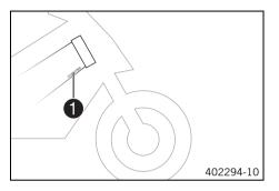
The chassis number 1 is stamped on the bottom right of the frame behind the steering head.
