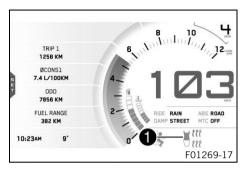
When the seat heating is switched on, the **Heated Seat** symbol appears in the **1** area of the display.
