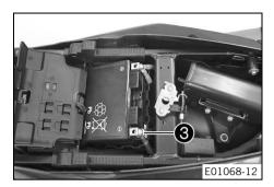
Connect both negative cables 3 to the battery.
