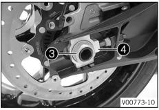
Remove nut 3. Remove chain adjuster 4.
