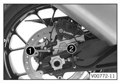
Remove screw 1 and pull wheel speed sensor 2 out of the hole.
