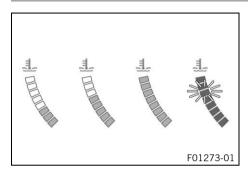
The coolant temperature indicator consists of bars. The more bars that light up, the hotter the coolant.
