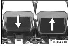
To move the combination instrument to the desired position, press the combination instrument upward or downward.
