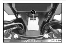
Socket **1** for electrical accessories is fitted in front of the upper triple clamp.
