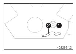
Remove screw 1 with the washers and take off shift lever 2.
