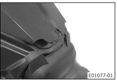
Raise the tank cover at the rear and take it off in a forward direction.
