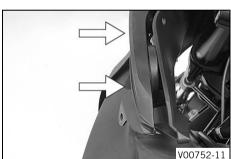
Position the mask spoiler and press laterally into the supports.
