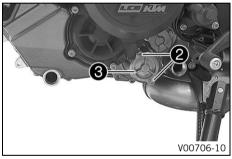
Remove screws 2. Remove oil filter cover 3 with the 0-ring.
