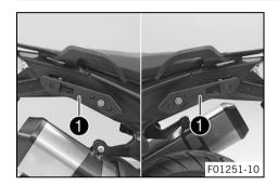
The case holders **1** are located on each side of the passenger seat.
