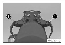
The passenger can hold onto grab handles **1** during the trip.
