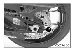
Push the wheel spindle in all the way and mount chain adjuster 4 and nut 5.
