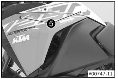
Mount and tighten screws **5**.
