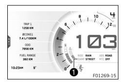
The **Damping** mode setting is shown in the **1** area of the display. The damping can be configured in the **Damping** menu.
