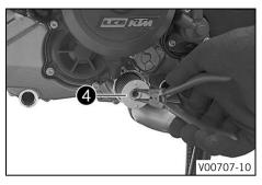
Pull oil filter **4** out of the oil filter housing.
