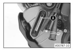
Add engine oil to the upper marking (A) on the engine oil level viewer.
