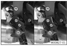
Adjust the footrest bracket to the desired position.
