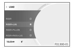
Settings for different loading conditions can be selected in the **Load** menu. A selection can be made between one-person operation, one-person operation with luggage, two-person operation, and two-person operation with luggage. The loading condition selected last is shown in the display.
