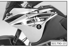
Mount and tighten screws 6.
