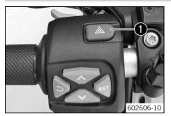
The hazard warning flasher switch **1** is fitted on the combination switch on the left.
