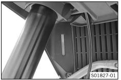
Add coolant until the coolant reaches the specified level.
