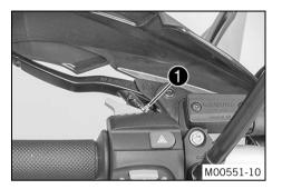
Adjust the basic setting of the clutch lever to your hand size by turning adjusting screw ①.
