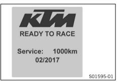
The matrix display is controlled using the menu switch ( p. 34). After the ignition is switched on, the display shows when the next service ( p. 60) is due.
