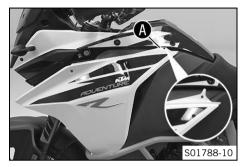
Position the side cover in the area A under the tank cover.
