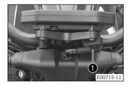
Plug in the connector 1 with sleeve.
