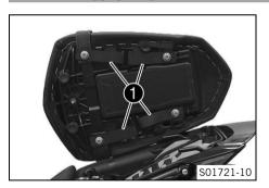
The baggage lugs **1** are located on the bottom of the passenger seat.
