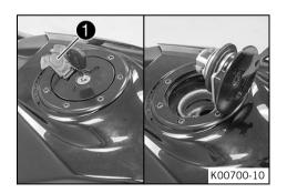
Lift the cover  ${\ensuremath{\bigodot}}$  of the filler cap and insert the ignition key in the lock.
