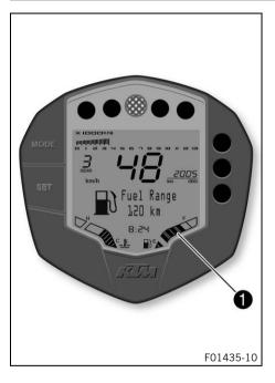
The fuel tank contents are shown in area **①** of the display. The fuel level indicator consists of bars. The more bars are lit, the more fuel is in the fuel tank.
