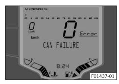
If an error has occurred in the CAN bus, various warning notes appear on the display: CAN FAILURE, CAN ABS FAILURE and CAN EMS FAILURE can occur.
