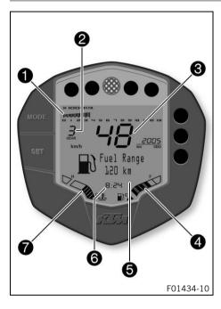
The tachometer ① shows the engine speed in revolutions per minute. The gear display ② shows the engaged gear. Speed ③ is shown in kilometers per hour km/h or in miles per hour mph. The fuel level display is displayed in the ④ area.
