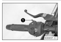
The high beam flasher button **1** is fitted on the left side of the handlebar.
