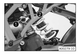
Turn adjusting screw ① all the way anticlockwise with a socket wrench.
