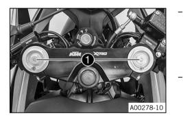
Turn adjusting screws 🕕 clockwise all the way.
