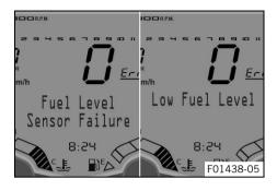
**Fuel Level Sensor Failure** appears on the display if the fuel level indicator is faulty.
