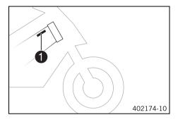
The vehicle chassis number **1** is stamped on the frame behind the steering head on the right.
