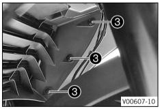
Remove expanding rivet 🕄.
