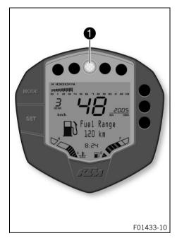
The shift warning light ① is located in the center above the display.
