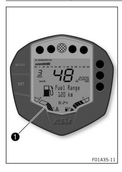
The coolant temperature display is shown in segment **1** of the display.
