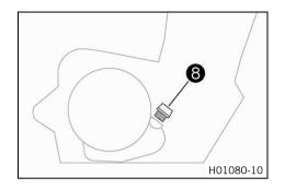
Remove filler plug (3) from the clutch cover together with the O-ring, and fill up with engine oil.
