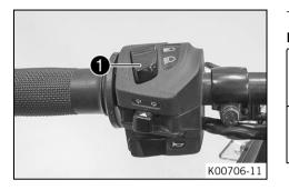
The light switch **①** is fitted on the left side of the handlebar.
