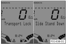
$\ensuremath{\mbox{Transport Lock}}$  appears on the display if transport mode is activated.
