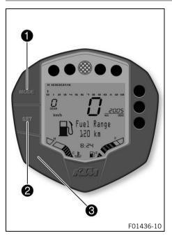
Press the **MODE** button ① to change display modes. Possible display modes are **TRIP F** (after reaching the fuel reserve level), **Error**, total distance traveled (**ODO**), distance 1 (**TRIP 1**) and distance 2 (**TRIP 2**).
