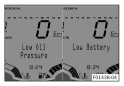
Low Oil Pressure appears on the display if the oil pressure is too
