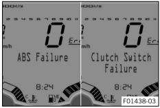
**ABS Failure** appears on the display if the ABS is no longer active. **Clutch Switch Failure** appears on the display if the clutch switch is faulty.
