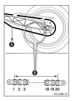
Pull the lower chain section with specified weight (A).
