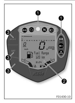
The combination instrument is attached in front of the handlebar.
