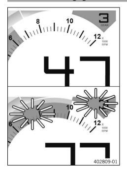
The shift warning light is integrated in the tachometer display. In the **Shift Light** menu, the engine speed for the shift warning light can be set. The shift warning light is always active during the running-in phase (up to 1,000 km / 621 mi). The shift warning light can only be deactivated, and the values for **RPM1** and **RPM2** can only be adjusted after this. The shift warning light lights up red at **RPM1** and flashes red at **RPM2**.
