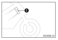
The chassis number **1** is stamped on the right side of the steering head.
