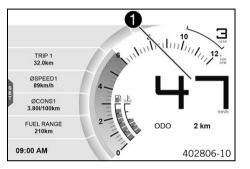
Speed **1** is shown in kilometers per hour **km/h** or in miles per hour **mph**.
