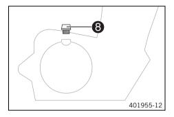
Remove filler plug 8 from the clutch cover together with the
