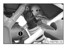
Adjust the spring preload by turning adjusting ring 1. Guideline
