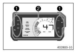
The combination instrument is attached in front of the handlebar. The combination instrument is divided into two function areas.
