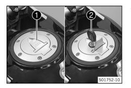
Lift cover lacksquare of the filler cap and insert ignition key m 2 in the fuel tank lock.
