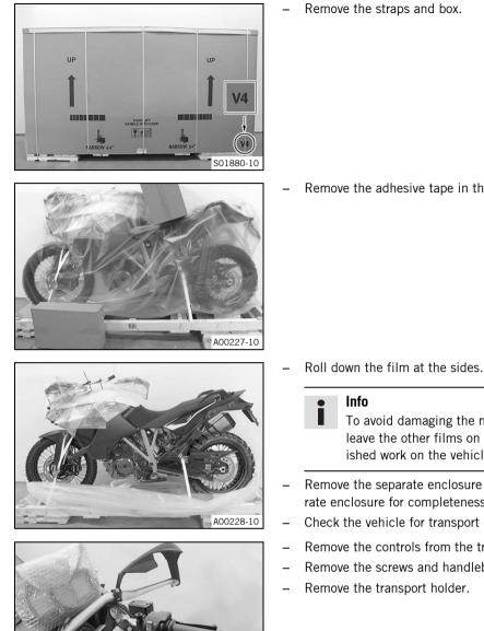
Remove the adhesive tape in the upper area of the motorcycle.
