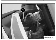
Turn the oil tank cap **1** counterclockwise and pull it up.
