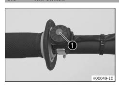
Kill switch **1** is fitted on the left side of the handlebar.
