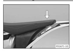
The seat engages with an audible click.Finally, check that the seat is correctly locked.
