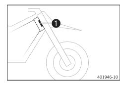
The type label **1** is located on the front steering head.
