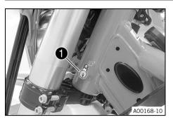
Steering lock **1** is fitted on the left side of the steering head. The steering lock is used to lock the steering. Steering, and therefore riding, is no longer possible.
