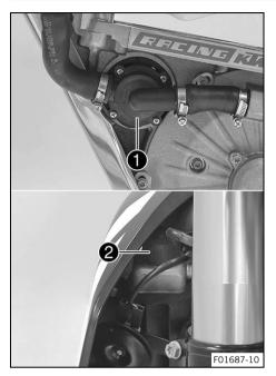
When the vehicle is in standby mode, the water pump **1** pumps the coolant through the cooling circuit.
