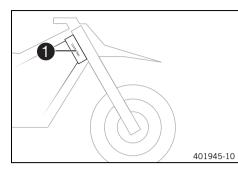
The vehicle identification number **1** is stamped on the right side of the steering head.
