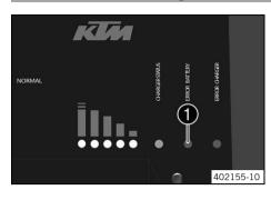
The faults are indicated by LED **1** on the battery charger. All of the following blink codes are displayed on the charger and refer to the KTM PowerPack.
