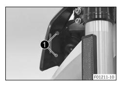
Push the release lever ① in the direction of the arrow. Lift the seat and fold it up.
