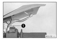
Adjust the free travel of the front brake lever using adjusting screw **1**.
