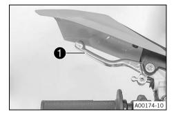
Rear brake lever 1 is fitted on the left side of the handlebar.
