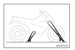
Use tension belts or other suitable devices to secure the motorcycle against falling over or rolling away.
