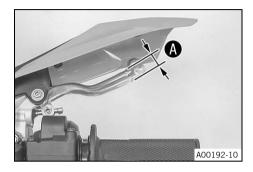
Push the front brake lever to the handlebar and check free travel  $oldsymbol{A}$ .
