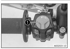
The light switch **1** is fitted on the left side of the handlebar. **Possible states**
