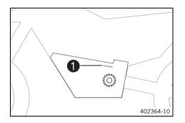
The motor number **1** is located on the left side of the motor over the motor sprocket.
