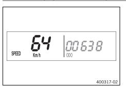
The current speed is displayed in the  $\ensuremath{\text{SPEED}}$  display mode. The current speed can be displayed in  $\ensuremath{\text{Km/h}}$  or  $\ensuremath{\text{Mph}}$ .
