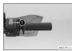
The main switch ① is attached to the right side of the handlebar. The main switch is also used as an emergency OFF switch. **Possible states**
