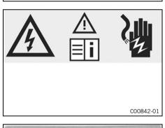
High-voltage components and electric shock, see the Owner's Manual
