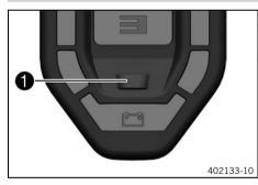
The driving mode tip switch **1** determines the driving mode. **Possible states**
