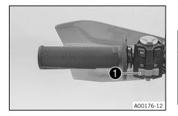
Turn signal switch ① is fitted on the left side of the handlebar.
