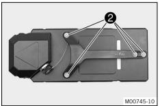
Install new charging socket ③ protection cap.
