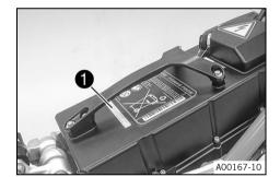
The battery identification number  $(\underline{BIN})$  (1) is stamped under the handle of the KTM PowerPack.
