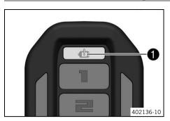
The errors are indicated by the yellow malfunction indicator lamp 1 and by acoustic signals that sound at the same time.
