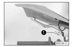
Adjust the free travel of the rear brake lever using adjusting screw **①**.
