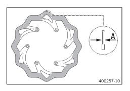
Check the front and rear brake disc thickness at multiple points for the dimension  $\mathbf{A}$ .
