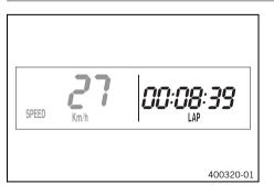
In the  $\ensuremath{\text{LAP}}$  display mode, up to 10 lap times can be timed with the stop watch.
