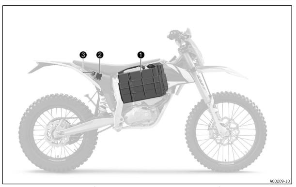
A rechargeable lithium-ion battery ① (KTM PowerPack, 260 V) and a 12 V battery ② are installed in the vehicle. The 12 V battery is located at the rear, under the seat. The fuse box ③ is located next to the 12 V battery. The KTM PowerPack is located under the seat and is bolted to the electric motor. The KTM PowerPack can be removed with just a few simple steps.
