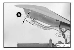
Push the rear brake lever to the handlebar and check free travel  $oldsymbol{A}$ .
