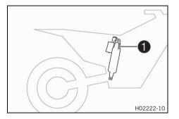
Shock absorber article number ① is stamped on the top of the shock absorber above the adjusting ring towards the motor side.
