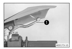
Front brake lever **1** is fitted on the right side of the handlebar.
