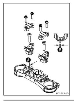
On the upper triple clamp, there are two holes at a distance of  ${f A}$  to each other.
