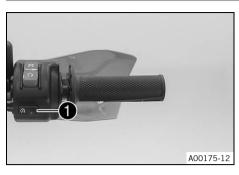
The start button **1** is fitted on the right side of the handlebar. The start button is only enabled when the main switch is switched on.
