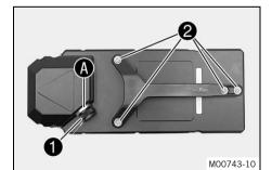
Remove ① charging socket protection cap.
