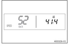
**A2** (average speed 2) shows the average speed on the basis of the current speed if the stop watch **S2** (stop watch 2) is running.
