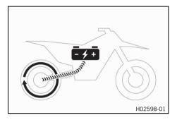
In the driving mode 1 (Economy) (IP p. 24), the KTM PowerPack is charged by the electric motor when the throttle grip is fully closed in overrun.
