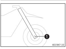
The fork part number **1** is stamped on the inner side of the axle clamp.
