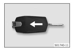
Fit lower half of the Race-on key and snap into place in the direction of the arrow.
