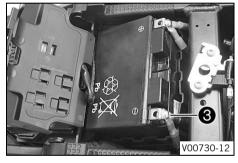
Disconnect both negative cables 3 of the 12-V battery to avoid damaging the onboard electronics.
