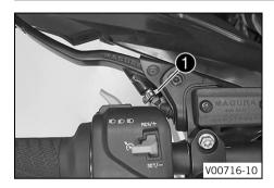
Adjust the basic position of the clutch lever to your hand size by turning adjusting screw ①.
