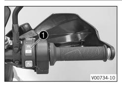
The emergency OFF switch/electric starter button 1 is fitted on the right side of the combination switch.
