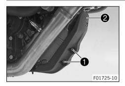
Remove screws 1 with bushings and engine guard 2.
