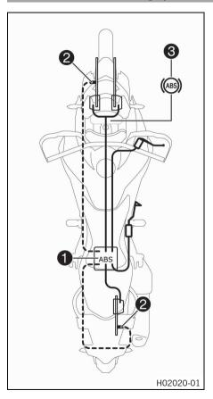
The ABS module ①, consisting of a hydraulic unit, brake electronics control unit, and a return pump, is located under the seat. One wheel speed sensor ② is located in each case on the front and the rear wheel
