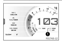
The ABS mode setting is shown in the **1** area of the display. The **ABS** can be configured in the **ABS** menu.
