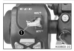
The cruise control system tip switch **1** is fitted on the left side of the combination switch.
