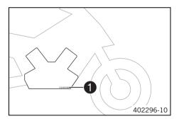
The engine number 1 is stamped on the right side of the engine.
