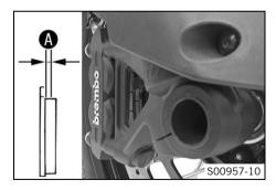
Check all brake linings on both brake calipers to ensure they have the minimum thickness (A).
