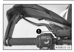
Adjust the basic position of the clutch lever to your hand size by turning adjusting screw 1.
