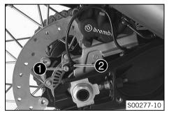
Remove screw 1 and pull wheel speed sensor 2 out of the hole.
