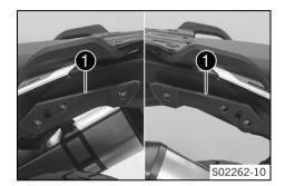
Case holders are located on each side of the passenger seat. A case system (optional) can be attached on the case holders. Use case systems approved and/or recommended by KTM. Observe the specifications in the enclosed **KTM PowerParts** fitting instructions.
