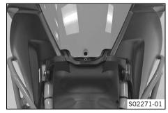
Raise the fuel tank cover at the rear and take it off in a forward direction.
