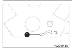
The shift lever **1** is fitted on the left side of the engine.
