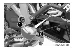
Check the chain sliding guard for wear at the recess.
