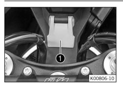
Socket **1** for electrical accessories is fitted in front of the upper triple clamp.
