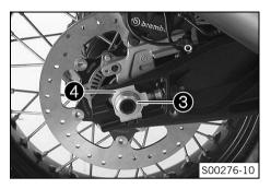
Remove nut 3. Remove chain adjuster 4.
