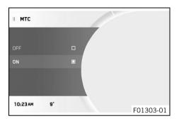
The motorcycle traction control ( $\underline{\mathsf{MTC}}$ ) lowers the engine torque in case of loss of traction in the rear wheel. Depending on the motorcycle traction control setting, a slight slip on the rear wheel may be desirable. Example: offroad.
