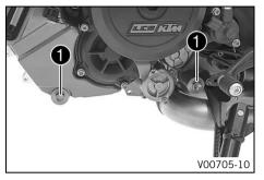
Mount and tighten oil drain plugs with the magnets, O-rings, and oil screens.
