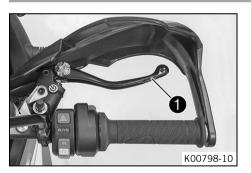
The hand brake lever **1** is located on the right side of the handlebar.
