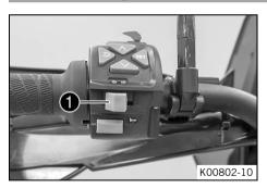
Turn signal switch **1** is fitted on the combination switch on the left.
