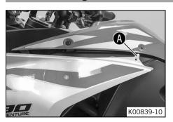
Position the side cover in area A under the fuel tank cover.
