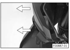
Remove the mask spoiler laterally from the supports.
