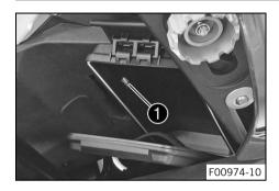
A USB socket 1 is located in the storage compartment for supplying power to external devices.
