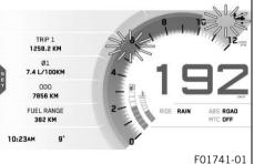
The shift warning light is integrated in the tachometer display. In the **Shift Light** menu, the engine speed for the shift warning light can be set. The shift warning light is always active during the running-in phase (up to 1,000 km / 621 mi). The shift warning light can only be deactivated, and the values for **RPM1** and **RPM2** can only be adjusted after this. The shift warning light lights up red at **RPM1** and flashes red at **RPM2**.
