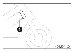
The vehicle identification number **1** is stamped on the bottom right of the frame behind the steering head.
