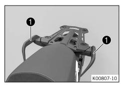
The passenger can hold onto the grab handles **1** during the trip.
