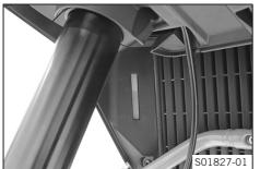
Add coolant until the coolant reaches the specified level.
