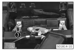
Connect both negative cables 3 to the 12-V battery.
