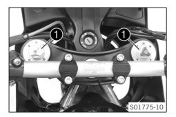
Turn adjusting screws **①** counterclockwise all the way.
