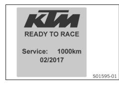
The matrix display is controlled using the <u>menu switch</u> (IP p. 33). After the ignition is switched on, the display shows when the next service (IP p. 59) is due.
