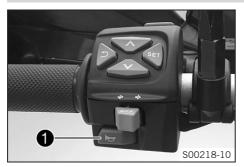
The horn button  $\ensuremath{\textcircled{0}}$  is fitted on the combination switch on the left.
