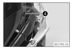
Pull the mask spoiler upward from bracket  $oldsymbol{4}$  .
