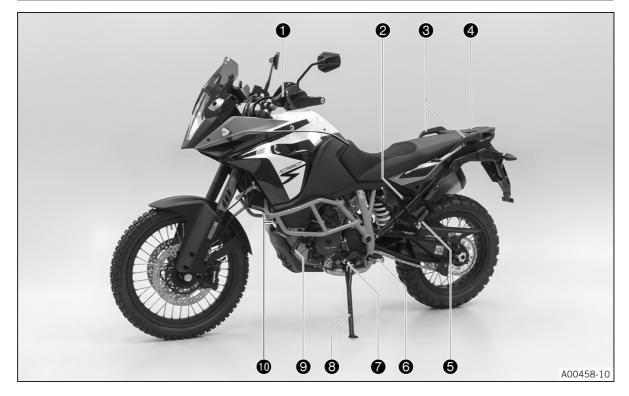
0 Clutch lever (🕮 p. 29) 2 Seat lock (🕮 p. 44) Grab handles (🕮 p. 45) 4 Luggage rack plate (🕮 p. 45) Passenger foot pegs (📖 p. 47) 6 6 Rider footrests (🕮 p. 81) **7** Shift lever () p. 47) 8 Side stand ( p. 49) 9 Engine oil level viewer 10 Fuel cocks (🕮 p. 43)
