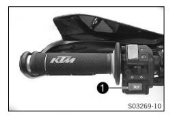
The horn button **①** is fitted on the left side of the handlebar.
