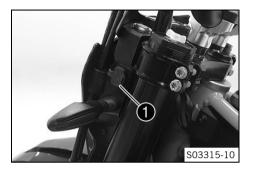
A USB socket ① for supplying power to external devices is located on the left side of the headlight mask. The USB socket is activated when the ignition is switched on.
