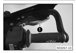
The hand break lever **1** is fitted on the right side of the handlebar.
