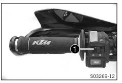
The turn signal switch  $\bigcirc$  is fitted on the left side of the handlebar.
