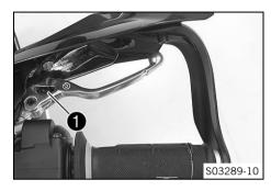
Adjust the basic position of the hand brake lever to your hand size by turning adjusting wheel ①.
