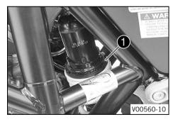
Adjust the spring preload by turning adjuster ①.
