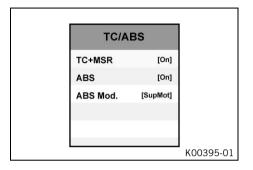
The traction control ( $\underline{TC}$  ( $\blacksquare$  p. 186)) lowers the engine torque in case of loss of traction in the rear wheel. Depending on the traction control setting, a slight slip on the rear wheel may be desirable.
