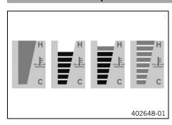
The temperature indicator in the display consists of 8 bars. The more bars that light up, the hotter the coolant.
