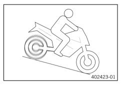
The  $\underline{\mathbf{MSR}}$  is an optional auxiliary function of the engine control. If the engine braking effect is too great, the  $\mathbf{MSR}$  prevents the rear wheel from locking.
