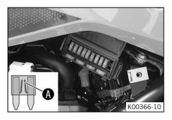
Remove the faulty fuse.
