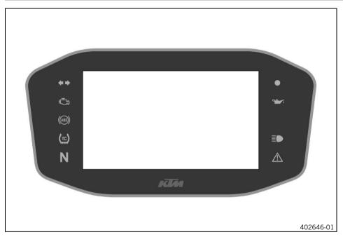
The indicator lamps offer additional information about the operating state of the motorcycle. When the ignition is switched on, all indicator lamps light up briefly.
