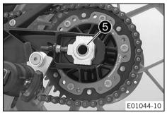
Pull out wheel spindle **5** far enough to allow the rear wheel to be pushed forward.
