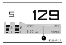
The current ambient temperature is shown in area **1** of the display.
