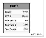
Press the UP or DOWN button until the "Trip 2" menu appears on the display.
