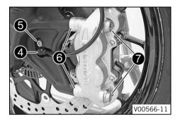
Position wheel speed sensor **4** in the hole. Mount and tighten screw **5**.
