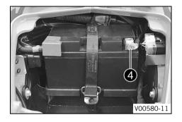
Connect negative cable 4 to the 12 V battery.
