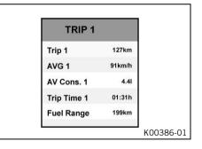
Press the **UP** or **DOWN** button until the "**Trip 1**" menu appears on the display.
