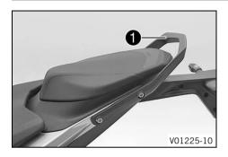
The grab handle 1 is used for maneuvering the motorcycle. If you carry a passenger, the passenger can hold onto the grab handles during the trip.
