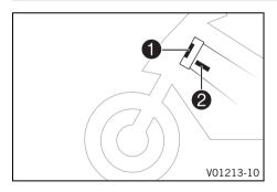
The type label 1 is located on the steering head on the left.
