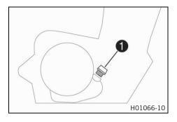
Mount and tighten filler plug with the O-ring.
