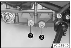
Mount the oil drain plugs 2 with magnets and new seal rings, and tighten.
