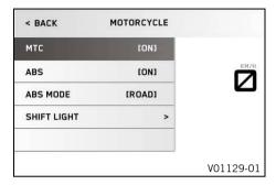
The motorcycle traction control (<u>MTC</u>) lowers the engine torque in case of loss of traction in the rear wheel.
