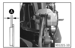
Check the brake linings for minimum thickness **A**.
