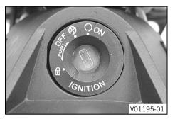
The ignition and steering lock is located in front of the upper triple clamp.
