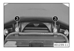
Mount and tighten screws 3.
