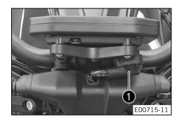
Plug in connector **1** with sleeve.
