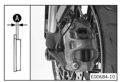
Check all brake linings on both brake calipers to ensure they have the minimum thickness **A**.
