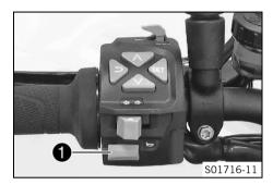
The horn button is fitted on the combination switch on the left
