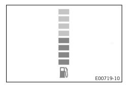
The fuel level indicator consists of bars. The more bars are lit, the more fuel is in the fuel tank.
