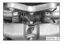
Loosen screw 3 using the hexagon socket wrench from the tool set.
