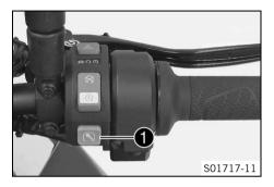
The <u>Race-on tip switch</u> is fitted on the right side of the combination switch.
