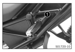
Seat lock 1 is located on the left side of the vehicle under the seat.
