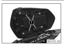
The baggage lugs **1** are located on the underside of the passenger seat.
