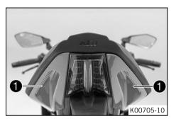
The grab handles **1** are used for moving the motorcycle around. If you carry a passenger, the passenger can hold onto the grab handles during the trip.
