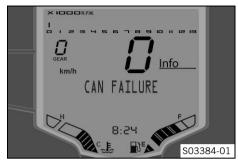
If an error has occurred in the CAN bus, various warnings appear on the display:
