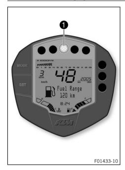
The shift warning light **1** is located in the center above the display.
