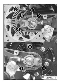
Pull the rear wheel back and mount wheel spindle **3** with the washer and chain adjuster **4**.
