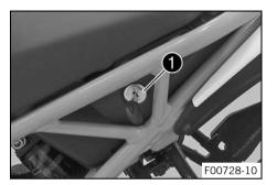
The seat lock **1** is located to the left of the seat. The seat lock can be unlocked using the ignition key.
