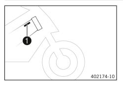
The type label **1** is on the right of the frame behind the steering head.
