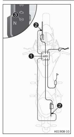
ABS unit ①, which consists of a hydraulic unit, ABS control unit, and return pump, is installed under the fuel tank. One wheel speed sensor ② is located in each case on the front and the rear wheel.
