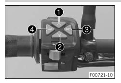
The menu switch is fitted in the middle of the left combination switch.
