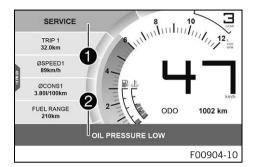
Warnings appear on the top and/or bottom edge of the display; these are marked yellow or red depending on their relevance. Yellow warnings 1 indicate errors or information which require prompt intervention or an adjustment to the riding style. Red warnings 2 indicate errors or information which require immediate intervention.
