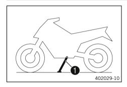
The side stand **1** is located on the left of the vehicle. The side stand is used for parking the motorcycle.
