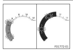
The shift warning light is integrated in the tachometer display. In the **Shift Light** menu, the engine speed for the shift warning light can be set. The shift warning light is always active during the running-in phase (up to 1,000 km / 621 mi). The shift warning light can only be deactivated, and the values for **RPM1** and **RPM2** can only be adjusted after this. In **RPM1** the shift warning light flashes and in **RPM2** it flashes and the color changes.
