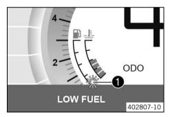
The fuel tank contents are shown in area **1** of the display. The fuel level indicator consists of bars. The more bars are lit, the more fuel is in the fuel tank.
