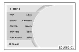
When the menu is closed, the Quick Selector 1 menu is opened by pressing the **UP** button.
