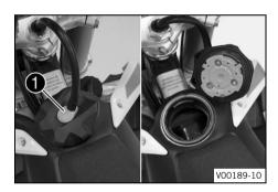
Press release button ①, turn the filler cap counterclockwise,
