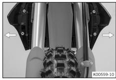
Pull both spoilers off the sides of the radiator bracket and lift off the fuel tank.
