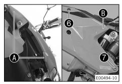
Mount and tighten screw with the collar bushing.
