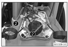
Detach plug-in connectors 2 and take off the headlight mask with the headlight.
