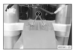
Mount and tighten screws 2.
