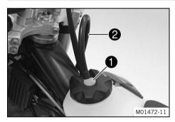
Mount fuel tank filler cap and turn it clockwise until the release button 1 engages.
