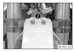
Mount and tighten screws 2.
