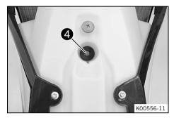
Remove screw 4 with the rubber bushing.
