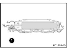
Position turn signal indicator lamp 1 in the combination instrument rack.
