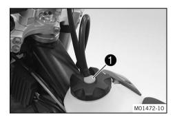
Press release button 1, turn the fuel tank filler cap counterclockwise, and lift it off.
