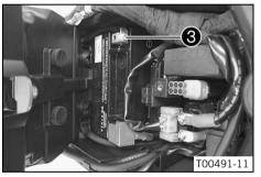
Disconnect negative cable 3 from the 12-V battery.
