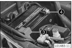
Position the positive cable and mount and tighten the screw. Guideline
