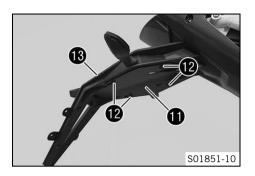
Mount splash protector with screws on license plate bracket
